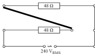
The elements needed to be connected in series as shown; however, many students connected them in parallel instead. Others added their own heaters into the circuit, showing no understanding of what the circuit represented.
