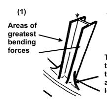
The forces are concentrated at the outer edges of the beam (1) thus this is where the largest amount of material needs to be located. (1)
