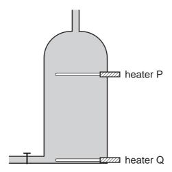
When only heater Q is switched on, it takes a long time to heat the tank of water to the required temperature of  $60\,^{\circ}$ C.
