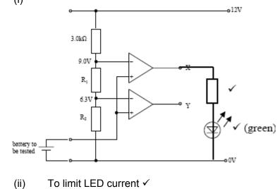
(iii) resistor voltage =  $12 - 2 = 10V\checkmark$ R = V ÷ I =  $10 \div 20mA\checkmark = 500\Omega\checkmark$  ecf
