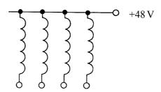
(b) The coils are operated by  $D_0$ ,  $D_1$ ,  $D_2$ ,  $D_3$  of the parallel port. The flow diagram below makes the test-tube rack rotate clockwise to the next test-tube i.e. 30°.
