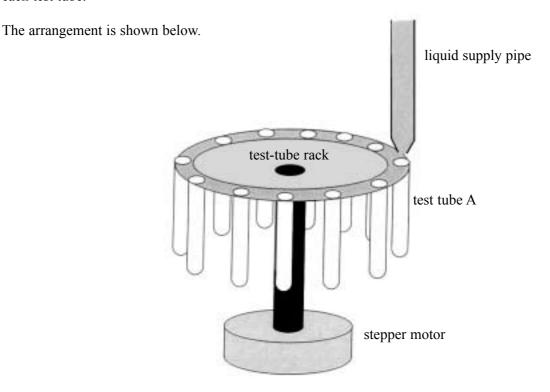
(a) The test-tube rack is rotated by a stepper motor. The stepper motor is 4 pole, operates from a 48 V supply and is controlled by a computer. The circuit diagram of the stepper motor is shown below.
