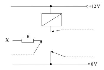
3 (a) (ii) Add to the diagram the component required to protect the transistor from the back emf of the relay.
