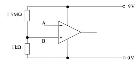
5 (c) (i) Calculate the voltage at point **B** in this circuit
