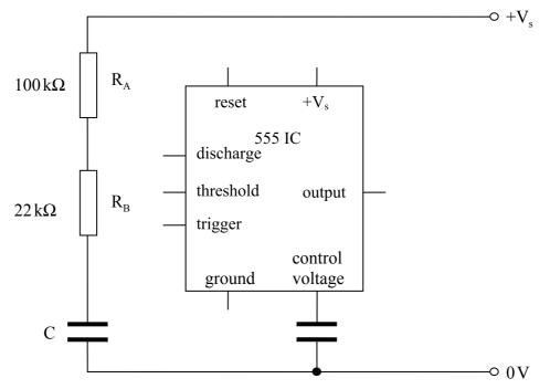
5 (d) (ii) Given the values shown on the circuit diagram for  $R_A$  and  $R_B$ , calculate the value of C required to give an output frequency of  $2\,\mathrm{Hz}$ .
