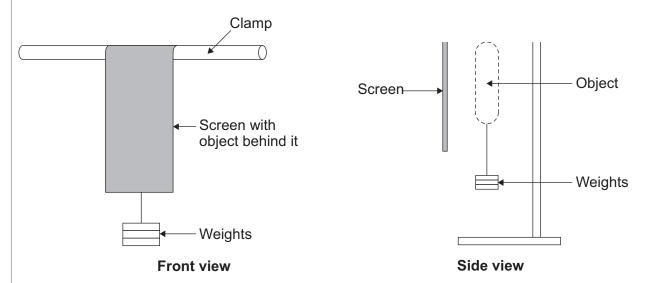
3 (a) Different weights are attached to the bottom of the object to exert different forces on it. In each case the extension of the object is measured. The table shows the results.
