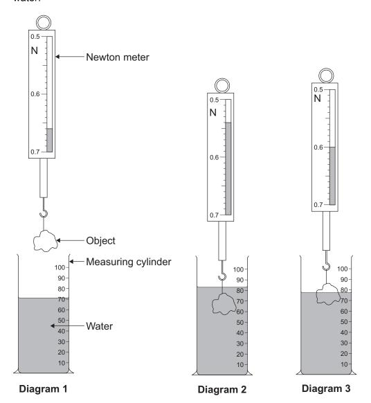
The table shows the readings taken from the newton meter and the measuring cylinder.
